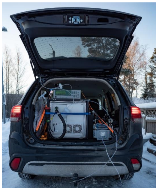
Figure 1: UiO's mobile laboratory with the PTR-TOF 1000 QB analyzer.
